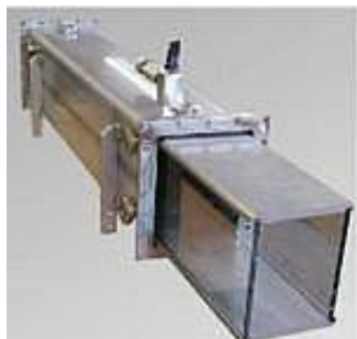
Neutron guide: Rectangular glass tube guiding neutrons by total reflection.
