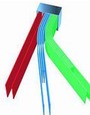
Horizontal splitting of the neutron beam.
