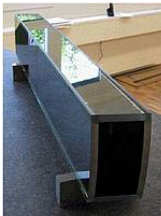
The coated glass of the neutron guide allows neutron guidance for more than 100m.
